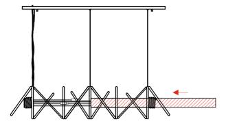
2 - Fix the fixing bar to the ceiling. (Screws not included. Please use screws suitable for the material of the roof).
