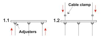
**3** - Connect the electrical wires; Fix the base with the metal buttons and adjust the steel cables with the desired lenght;
