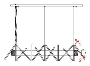
**6** - Put the metal box (ø60 with 40mm) in the same place as the beginning. Conclude with the metal piece .
